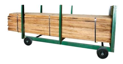
The Model 100-H is a heavy-duty one-piece lumber cart with rigid uprights. These units are fabricated with 2" x 6" structural steel tubing main rails, and the uprights are made with 2" x 4" structural steel tubing. Each cart is equipped with 12" x 3" phenolic wheels. They can be ordered in eight or ten foot lengths, or can be custom-made to your requirements.
