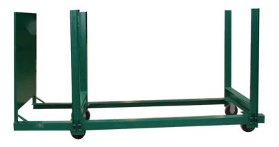
The Model 100-C is a heavy-duty one-piece lumber cart with limited pivoting uprights. The main frame is fabricated from 4" angle iron, and the uprights from 4" channel. They are equipped with 8" x 3" casters. When the bunk is full, the uprights can released and moved slightly off 90°, allowing the pack to be lifted out with no restrictions or hang ups.
